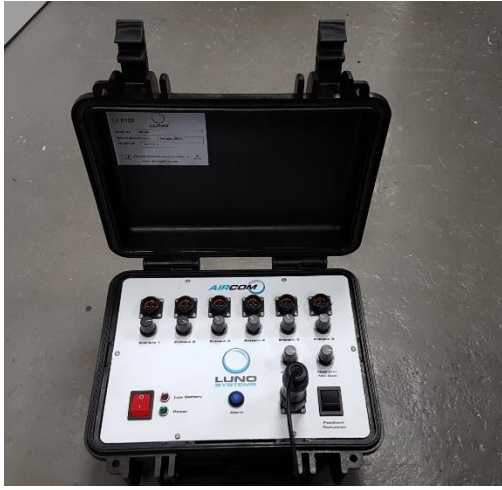
Main Aircom 6 control box
